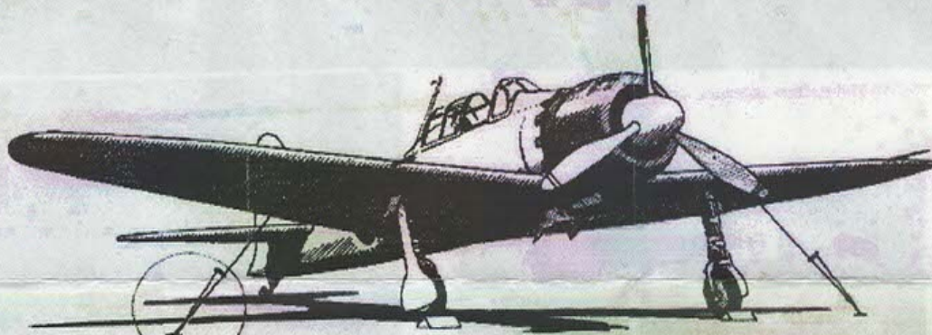
Typical tie down arrangement on an Imperial Japanese Navy Carrier
